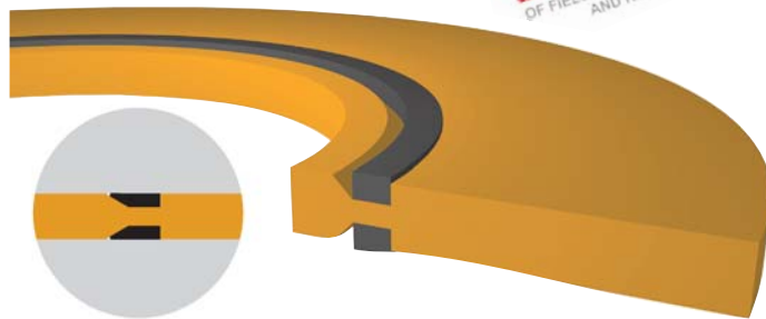
After Bolt Tightening
